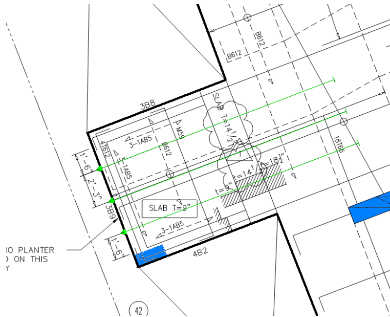
Figure 11: Cantilevered balcony utilizing post-tensioning
